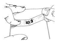
**Note:** Micro-Measurements PCT-2M gage installation tape must be used if tape is employed to position the gage. Other tapes may react with uncured adhesive.
